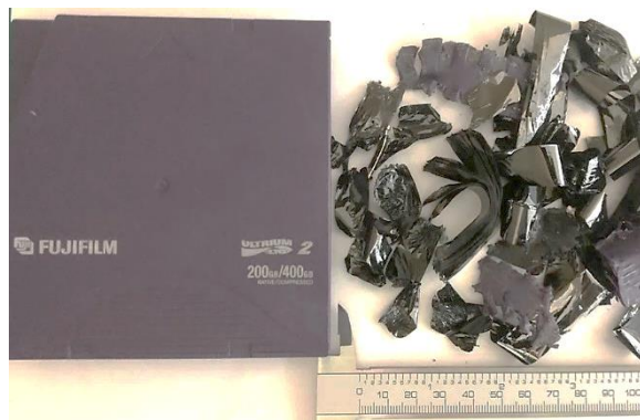
Magnetic Tape Disk DIN 66399-T2 (18 mm wide blade)
