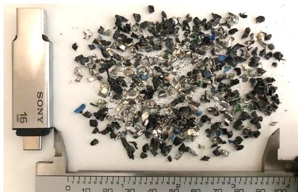
Thumb Drive 3-Stage Shred DIN 66399-E5 (2mm particle size)
