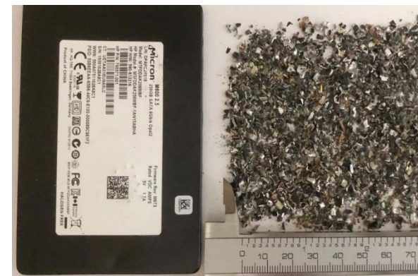
SSD 3-Stage Shred DIN 66399-E5 (2mm particle size)
